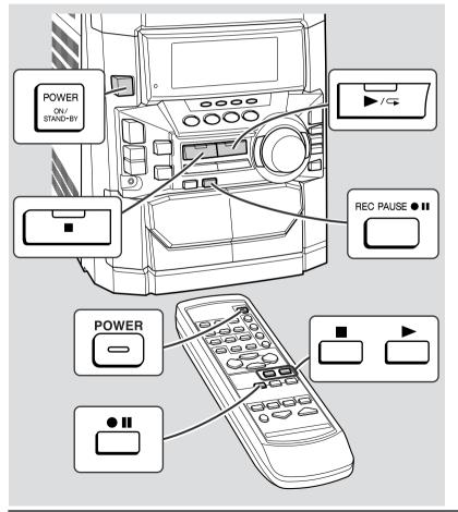
Recording can be operated in the TAPE 2 compartment. The TAPE 1 is for playback onlv.
